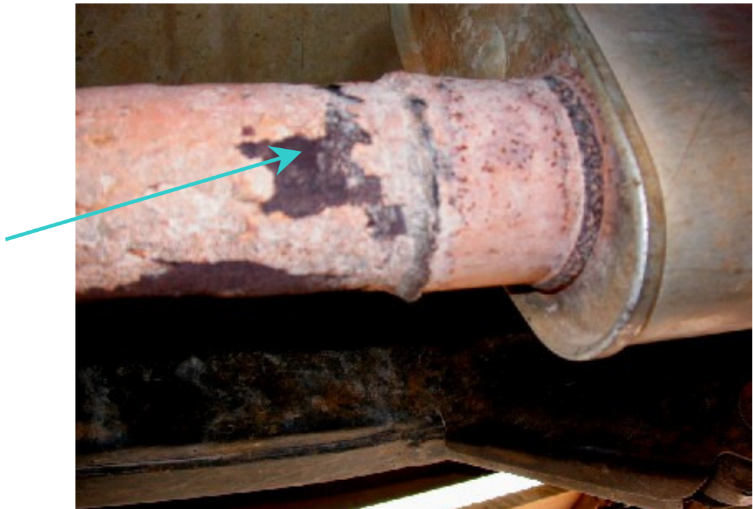
Figure 12 Location of leak on main exhaust pipe immediately adjacent front of non-standard muffler box (arrow). Note condition of weld and extensive corrosion deposit. This hole was used to locate thermocouple channel #5 in exhaust stream.
