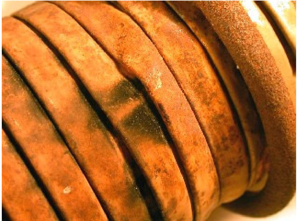
Figure 7 Detail of flexible tube showing carbon soot deposits associated with tube elements.
